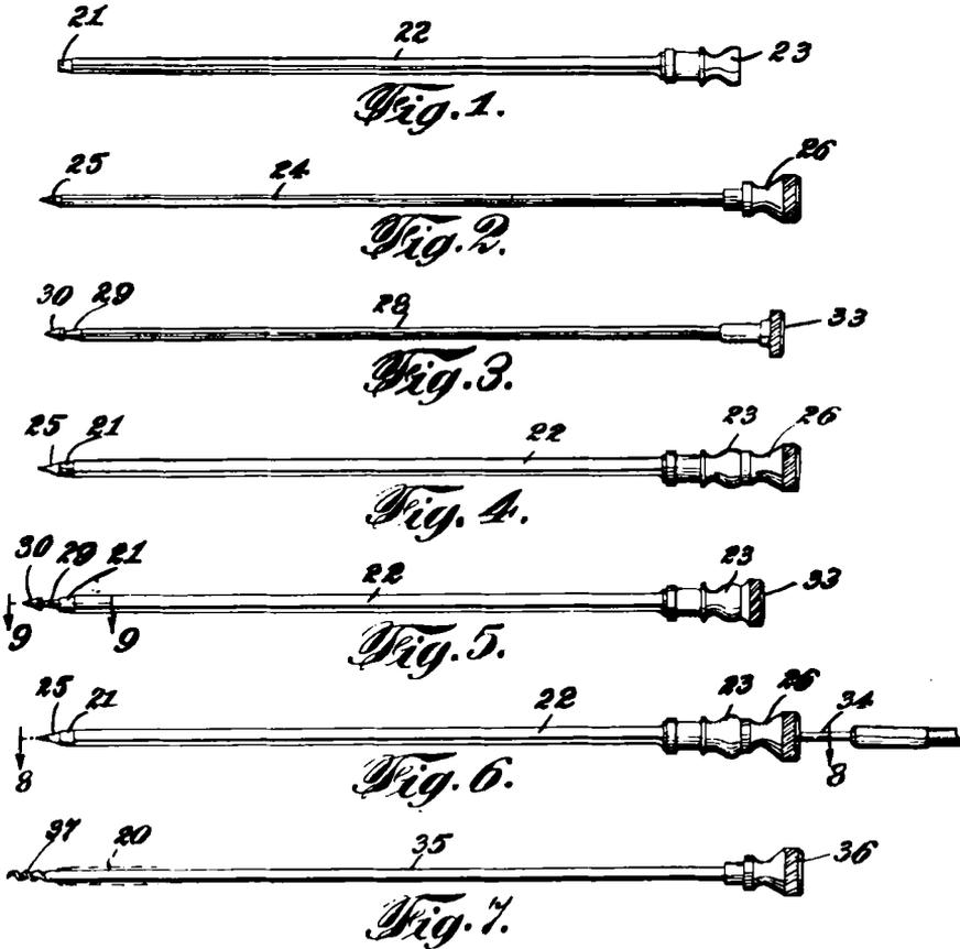
FIG. 1. INSULATED STEEL SHEATH. (21) cutting edge; (22) insulation; (23) syringe collar.
