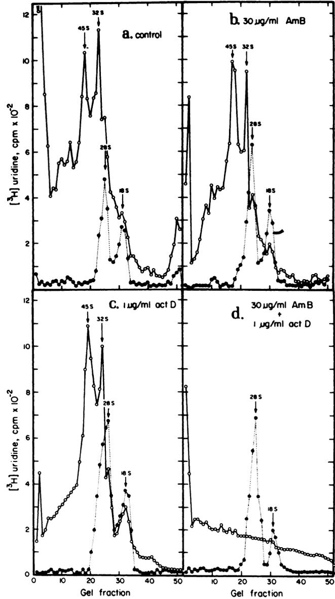
Chart 1. Acrylamide gel electrophoretic analysis of [ $^3$ H]uridine pulse-labeled RNA from untreated HeLa cells (a) and cells treated with AMB (AMB) (b) and actinomycin D (act D) (c) alone and in combination (d). The method of analysis is described in the text. (●) marker 18 S and 25 S RNA. (○) pulse-labeled [ $^3$ H]RNA.
