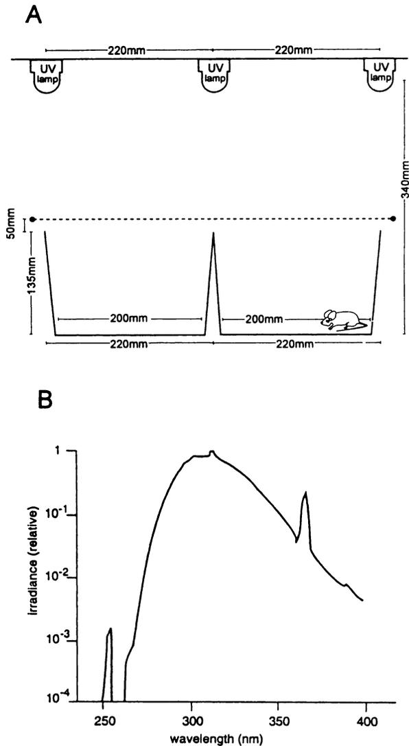
Fig. 1. A, scaled schematic representation of the exposure configuration. B, relative spectral energy output of the Philips F40 sunlamp.
