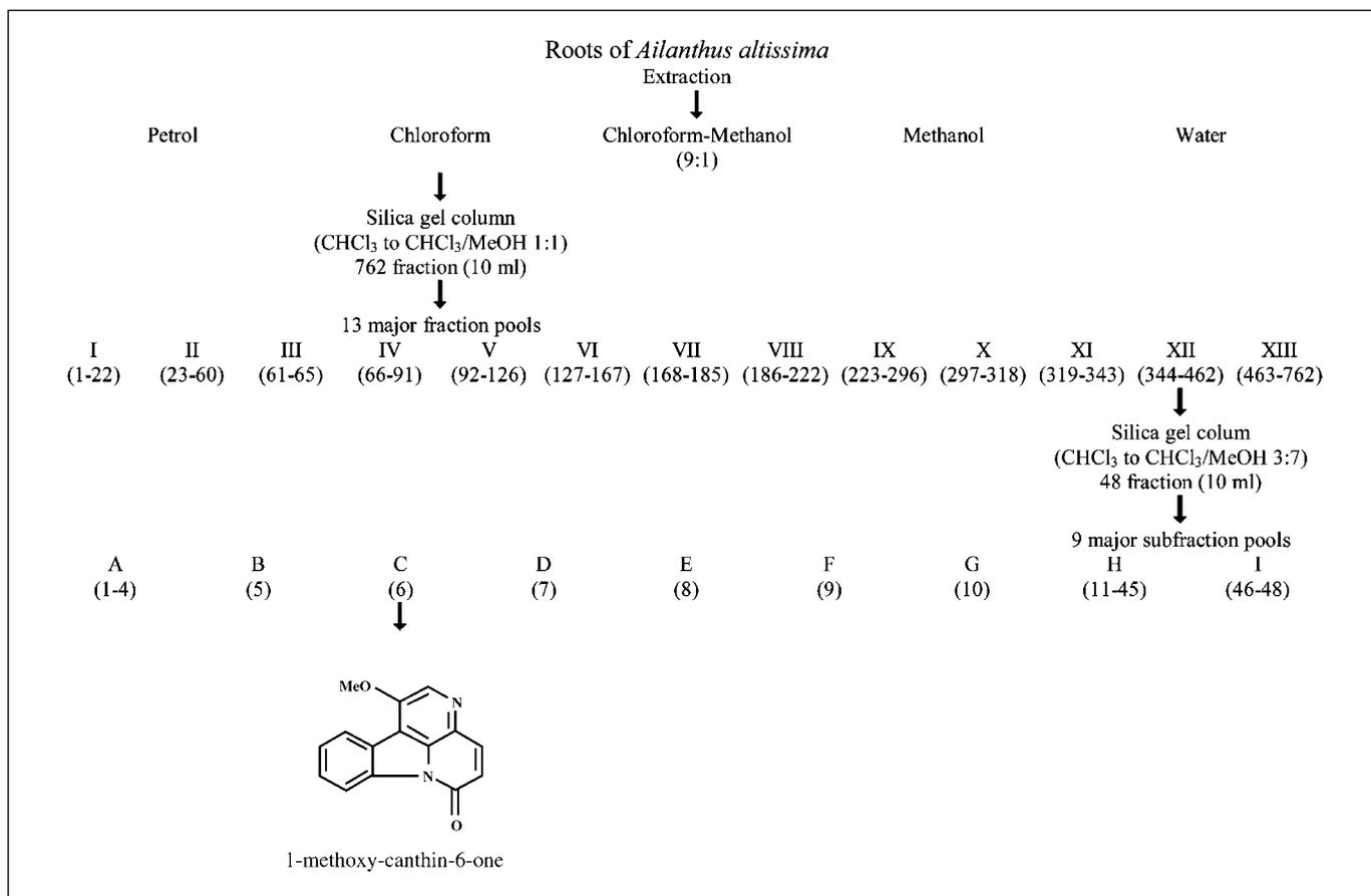
Figure 1. Extraction procedure for 1-methoxycanthin-6-one.
