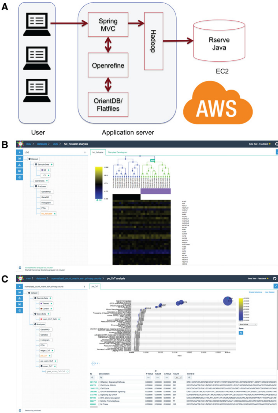
Figure 1. A , An overview of WebMeV's architecture. B and C , Screenshots of WebMeV showing a simple hierarchical clustering ( B ), and a bubble plot summarizing the results of a gene set enrichment analysis ( C ).
